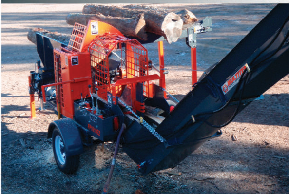
Optional 2-Strand Hydraulic Live Deck
