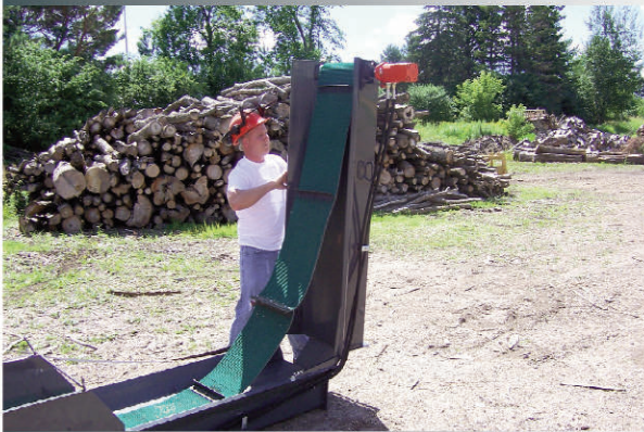
13' Folding Conveyor System
