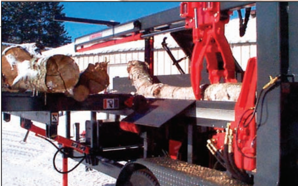
The unique shuttle-grapple makes it possible for you to efficiently produce firewood from low grade logs.
