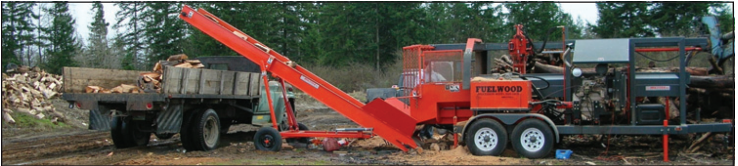
Gulley Logging firewood production operations with Multitek Model 2020LDS firewood processor.
