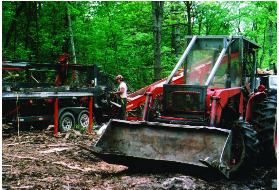
The Multitek easily cuts and splits 2 cords of wood each hour, filling the waiting truck with split wood that flows up the hydraulically run 30-foot stacking conveyor belt.
