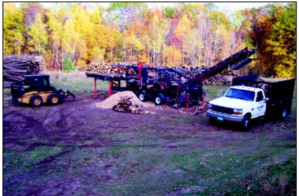
Multitek Model 2020CSC firewood processor is equipped with integrated stacking conveyor for easy top-loading of trucks.
