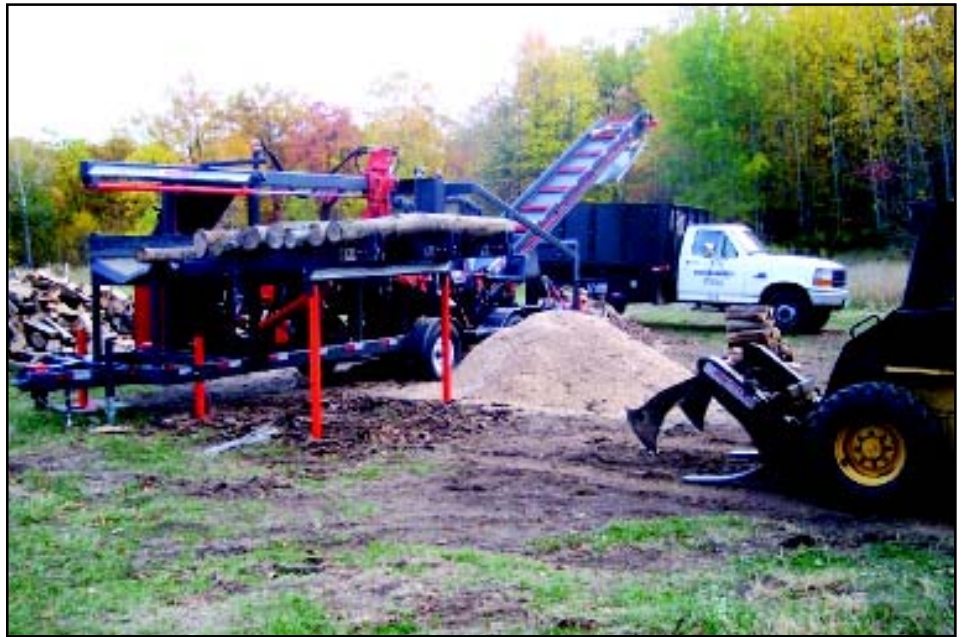
Multitek's exclusive in-feed shuttle grapple carriage, visible above logs, enables operator to process the most crooked logs.
