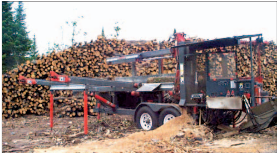
Wood yard at Malley Firewood with Multitek firewood processor model 2020LDCS and plenty of firewood logs.
